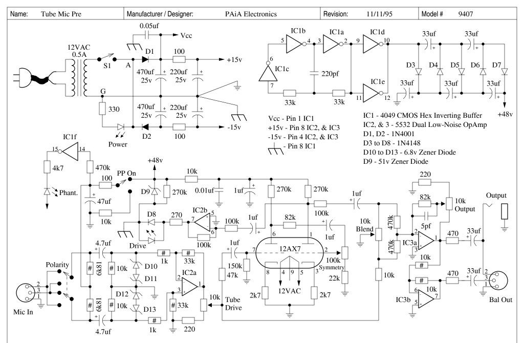
All 33uf caps 16v all others 50v unless marked othewise. Resistors marked with # are 1% film type. The "Drive" LED indicates how hard the tube is being driven. The "Blend" control allows for a mixing of SS and tube coloration. Symmetry controls the relative amounts of even and odd harmonics, CCW the Tube Mic Pre may sound punchier, while CW it may sound warmer. The 12VAC needed for pin 5 of the 12AX7 can be obtained from point G while pin 4 should be connected to point A.
